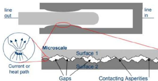
Fig. 3. Schematic view of the surface contact between two metals. [11]
