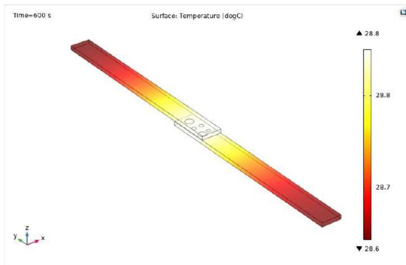
Fig.6. Temperature distribution in the contact zone and cooper strips.
