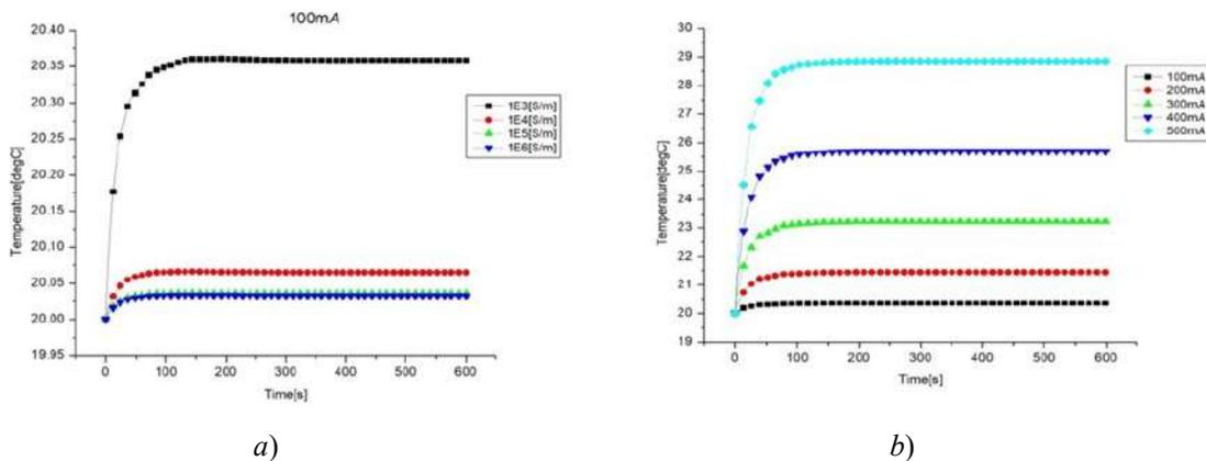
Fig.7. Temperature variation with time obtained by a point measurement at the interface of the overlapping conductors for: a) Different values of electric conductivity of the oxide film and an injected current of 100 mA; b) Different values of injected current.
