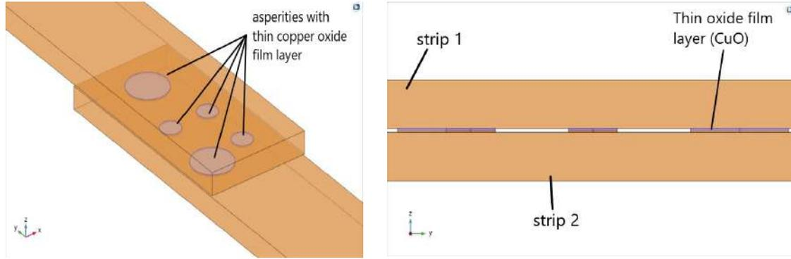
Fig.4. Geometrical model with copper oxide asperities.
