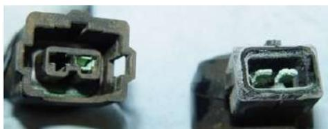
Fig.1 Corroded connector terminals. [8]
