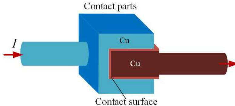
Fig. 2. Schematic view of electric contact.
