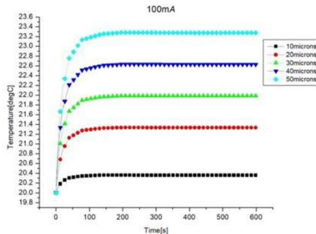
Fig.9. Temperature variation as a function of the oxide film thickness at the contact interface.
