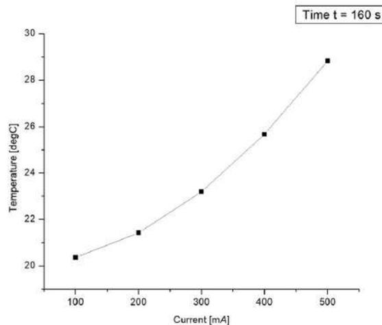
Fig. 8. Variation of steady state temperature as a function of injected current.
