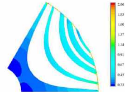
Fig. 10. SynRel motor with no radial ribs: flux density map at maximum speed [T].
