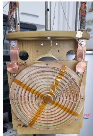
Fig. 12. Model experimental de limitator supraconductor HTS de tip rezistiv
